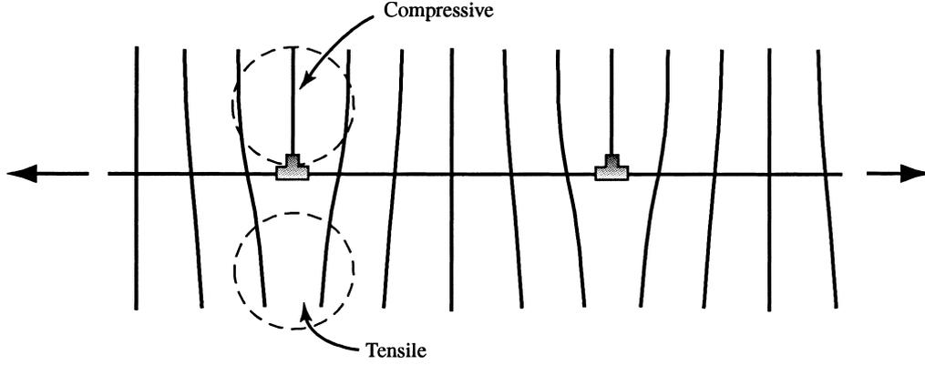
Fig. 3. Schematic diagram of the semi-coherent interface between Ag and Ni. Upon extension of the interface, the non-linearity of the elastic displacement field lowers the strain energy of the compressed regions more than it raises that of the tensile regions, resulting in a compressive contribution to the interface stress.
