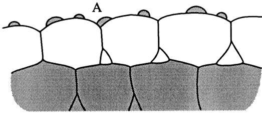
Fig. 13. Illustration of the renucleation that occurs at the start of the deposition of each layer in a multilayered film. Coalescence of these new islands leads to tensile stresses. Point A shows coalescence between a new island and a substrate grain; since this can happen early in the deposition process, there is no compressive transient.
