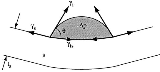
Fig. 6. Schematic diagram of the substrate curvature resulting from the force action of the surface and interface stresses associated with an isolated island. The dimensions have been exaggerated for clarity.
