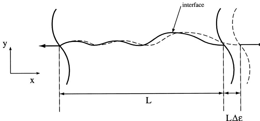
Fig. A1. Illustration of the deformation of a non-planar interface upon application of a strain  $\Delta\epsilon$ .
