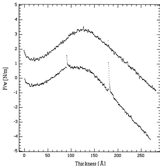
Fig. 5. Force-per-width curves measured during continuous (upper) and intermittent (lower) depositions of Cu. Time intervals between depositions are not shown. The data of the continuous deposition are offset by 2 N/m for clarity. The close similarity between the two curves demonstrates the reversibility of the changes upon interruption and resumption (see Fig. 7). From Ref. [19].
