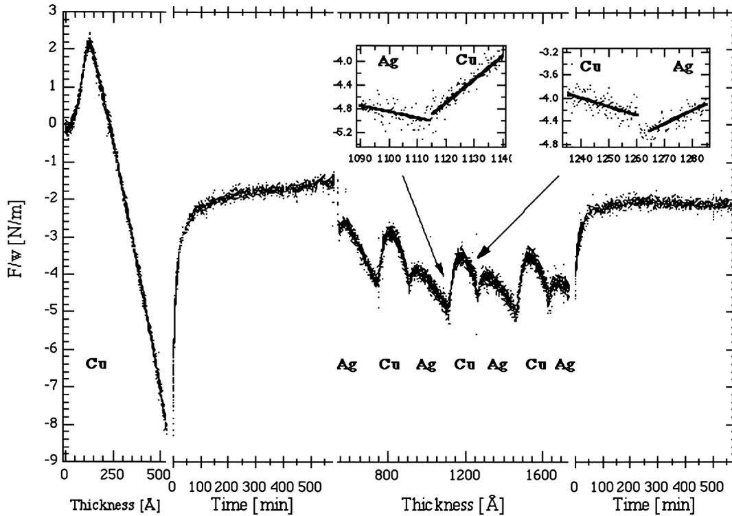
Fig. 12. Force-per-width curve measured during and after deposition of a multilayer. There was a pause after the deposition of the first layer (Cu). Subsequent layers were deposited continuously (no pauses). The tensile rises seen after each deposition switch are the result of renucleation (see Fig. 13). The insets show the discontinuities used to determine the Cu/Ag interface stress. From Ref. [19].
