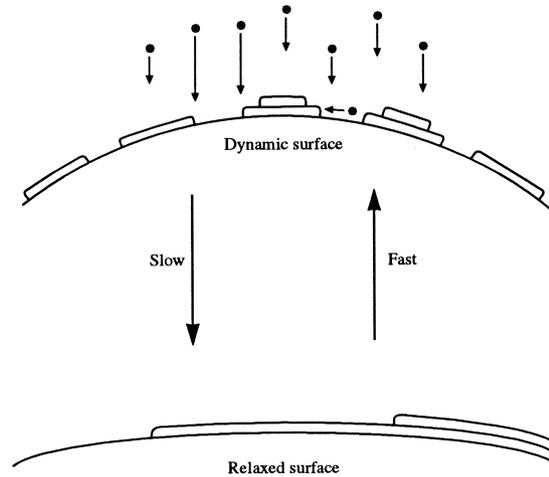
Fig. 8. Schematic diagram of the difference in surface stress between a dynamic surface and a relaxed one. The elimination of ledges makes the relaxed surface less compressive. The time constants changing the surface structure upon interruption and resumption of the deposition are different.
