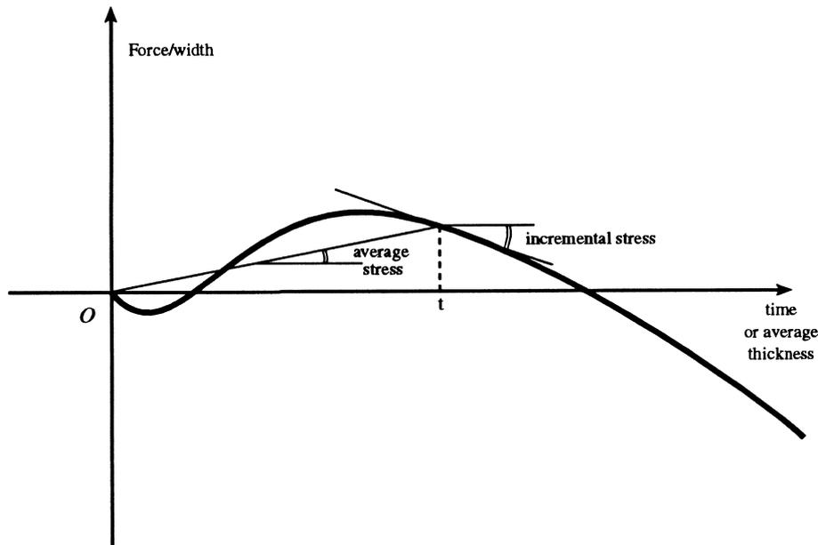
Fig. 4. Generic diagram of a force-per-width curve (proportional to curvature) measured as a function of time or effective thickness during vapor deposition. The average and incremental stresses at time or thickness  $t$  are indicated.
