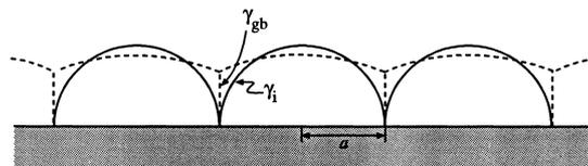
Fig. 10. Illustration of the Nix-Hoffman mechanism for generating tensile stresses by coalescence of individually nucleated islands. The island surfaces, with surface energy  $\gamma_i$ , come together to form a grain boundary with energy  $\gamma_{gb}$ .
