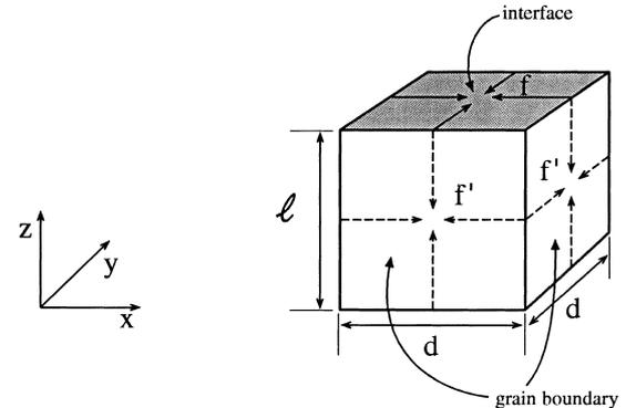
Fig. B1. Illustration of the interface and grain boundary stresses acting on an isolated grain in a layer of a multilayered film.
