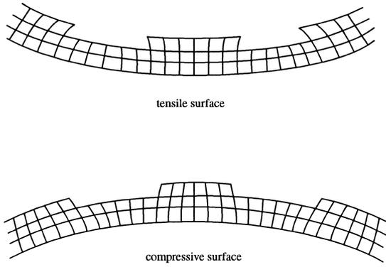
Fig. 1. Schematic illustration of how the next-nearest neighbor interactions of the atoms at the edges of a ledge can give tensile and compressive surface stresses.
