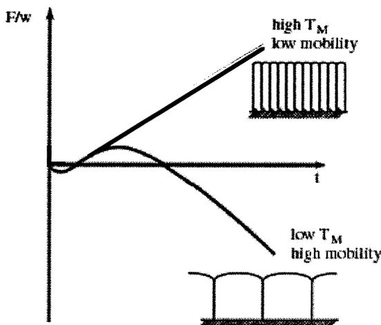
Fig. 9. Generic diagram of the force-per-width characteristic for high-mobility and low-mobility materials. The respective microstructures are indicated. After Abermann *et al.* [24-27].
