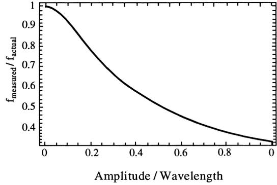
Fig. A2. The ratio of the measured to the actual interface stress for a sinusoidally shaped interface, as a function of the amplitude of the height variation.
